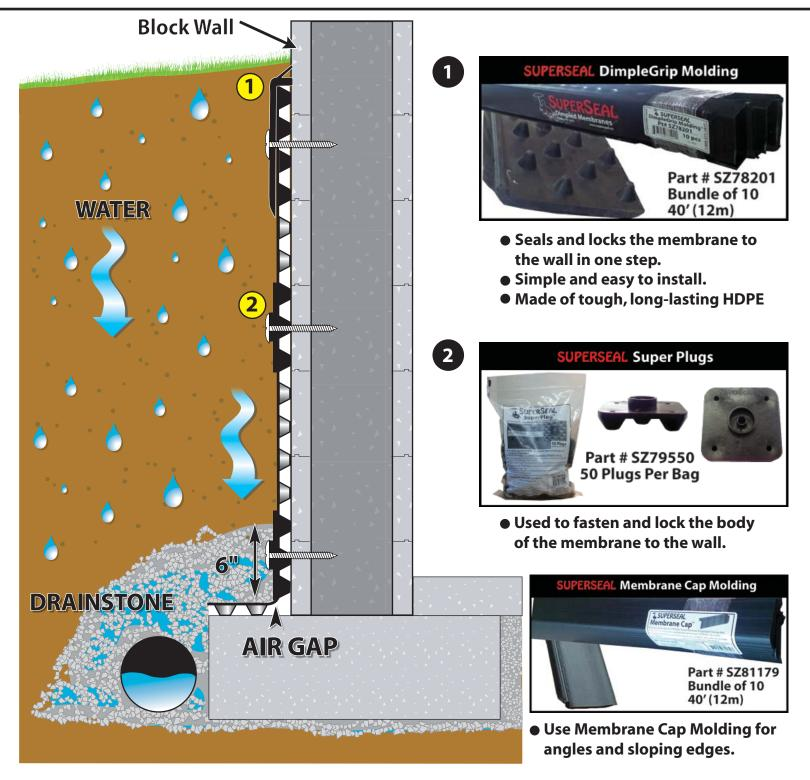
When installing SUPERSEAL Dimpled Membrane on a concrete block foundation, always use DimpleGrip Molding for the top and side edges and Super Plugs to fasten the body of the membrane to the wall.
