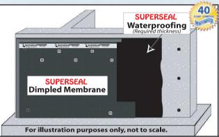
**SUPERSEAL** Dimpled Membrane protects the waterproof coating from backfill, removes 100% of the headwater pressure off the face of the wall, and creates a drainage space for moisture.
