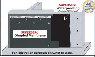
**SUPERSEAL** Dimpled Membrane protects the waterproof coating from backfill, removes 100% of the headwater pressure off the face of the wall, and creates a drainage space for moisture.
