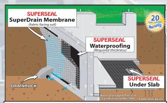
**SUPERSEAL** SuperDrain Membrane controls the flow of water providing drainage away from your foundation. This creates, dryer and lighter soil loads, and reduces the stress on your foundation.
